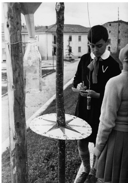
Figure 1. Students at a meteorology lesson: anemoscope. Photo print (12.9x18 cm) belonging to the Indire photographic heritage. The title is on the rear of the photo: “anemoscope”. Students of the “Iacobucci” Elementary School in Campobasso are at the Vinchiaturo (Campobasso) weather station to study an anemoscope: a device to measure the direction of winds.
